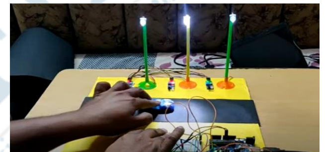
Fig. 6. As the car passes through the second LED the intensity of LED 2 increases and the intensity of LED 1 decreases
